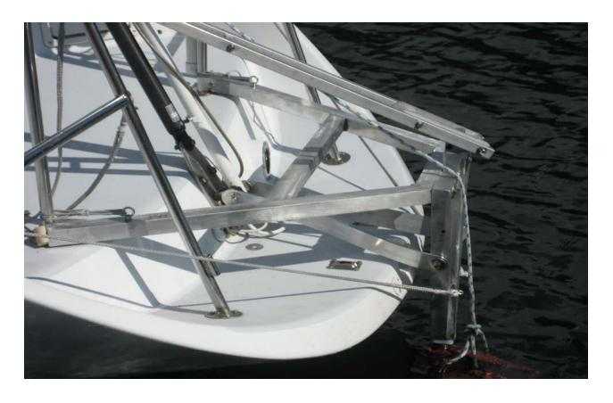
"Torsion loads on the frame were immense and caused the welds to fail. This was under power at < 3 knots"
